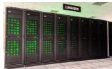
LONGHORN 104 node IBM Power9 based system 4 Nvidia V100 GPUs per node EDR Infiniband
